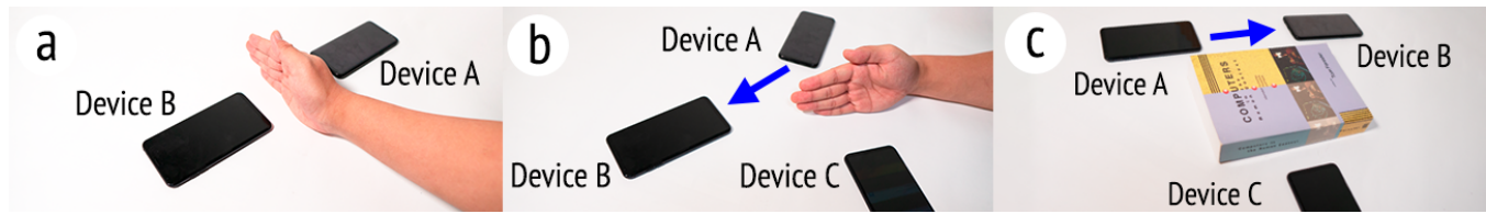
Figure 9: Hand action and everyday objects on a physical surface can play various roles for the Bit Whisperer communication: (a) a hand can block to stop communication between two devices and open up to restart the communication; (b) Access control can be managed by blocking the line of sound with a hand to share data selectively; (c) everyday object like a book can be an obtrusive shield to protect the communication between Device A and B from a sniffing attempt of Device C.
