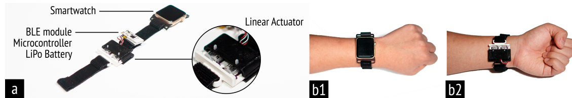
Fig. 1. Spidey Sense is a smartwatch wristband that produces squeezing sensations to alert people to “urgent” cybersecurity warnings. (a) The latest version of the Spidey Sense wristband, compatible with an Apple Watch. This version was developed after our evaluation. (b1) Top view of an Apple Watch with Spidey Sense; and (b2) Bottom view of an Apple Watch with Spidey Sense.
